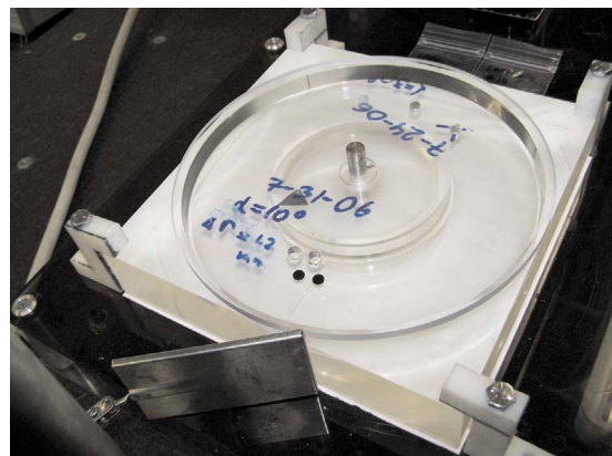
FIG. 1. (Color online) Closeup of the experimental arrangement showing the Couette cell covered with one of the acrylic templates used to deposit the particles and the 45^\circ mirror (bottom of the image).
