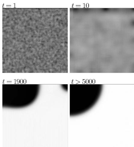
FIG. 4. Time series in  $(x, z)$  plane for the formation of a vapor bubble in a liquid ( $\bar{\rho}=0.83$ ). The boundary conditions for the density field at the solid walls favor the bubble to be in contact with the solid surface.
