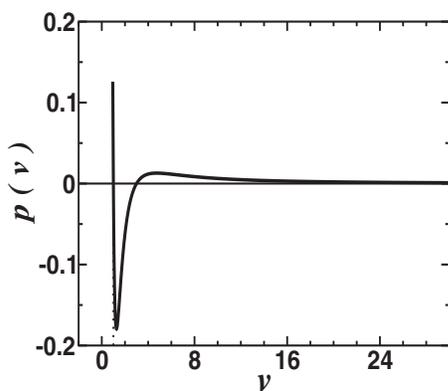
FIG. 1. The pressure corresponding to the free-energy density (5) as function of  $v=1/\rho$ . The unit volumes for liquid and vapor phase are  $v_l=1$  and  $v_v=\infty$ , respectively.
