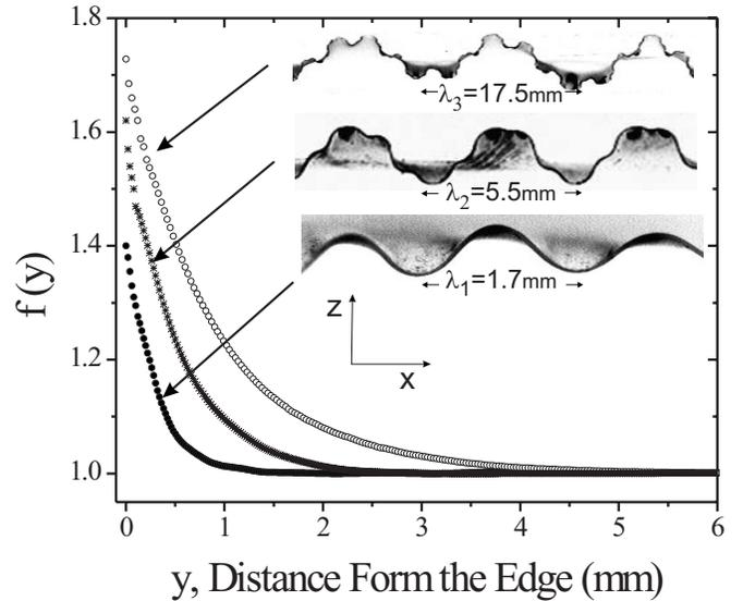
FIG. 2. Metric function describing the elongation in the  $x$  direction as a function of  $y$ , measured for 0.20-mm-thick polyethylene sheets for different conditions: top curve—crack velocity  $v = 0.5$  cm/s, steady state; middle— $v = 5$  cm/s, steady state; bottom— $v = 5$  cm/s, initial crack propagation. The resultant structures along the edge (inset) consists of three, two, and one generations, respectively.
