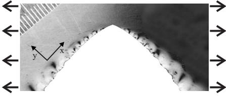
FIG. 1. A spade-shaped crack traveling in a polyethylene sheet that is pulled horizontally. The sheet edges created by the tearing have stable waves.  $y$  is the distance of a point from the edge, measured along the surface. The lines on the scale in the upper left corner are 1 mm apart.
