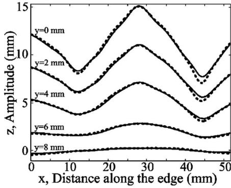
FIG. 4. Comparison of the amplitude as a function of  $x$  at different  $y$  for the full sheet (solid lines) with the amplitude measured after cutting off successive strips of 3 mm along the edge (dotted lines). The comparison shows that the wavelengths and amplitudes are not affected by the removal of the strips. The values of  $y$  were measured here in the laboratory frame with respect to the cut edge, rather than along the surface as in the rest of the measurements we present.
