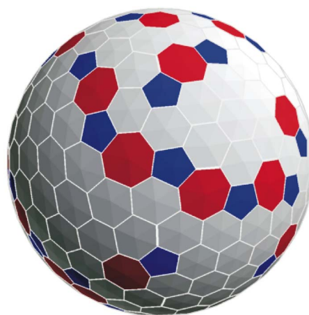
FIG. 5. (Color online) Voronoi diagram for the cylindrical phase on a sphere of radius R=20.0 , with f=0.8 and \chi N=25.0 . The sphere consists of 446 microdomains (69 fivefold, 350 sixfold, and 57 sevenfold coordinated sites) and exhibits grain boundary scars.
