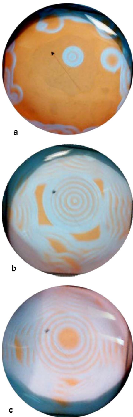
FIG. 1. (Color online) Behavior of a target located at 12.5 mm from the rotational center for different velocities of rotation (a) 30 rpm, (b) 50 rpm, and (c) 70 rpm. (The arrow in the figures is just a reference that shows the orientation of the Petri dish.)
