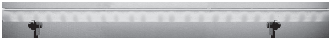
FIG. 2. Axial segregation pattern of a 50%:50% mixture of glass beads, after 20 min at 15 rpm. Dark areas represent bands of small particles; bright bands contain large particles at the surface. The width of the drum is \approx 1 m.
