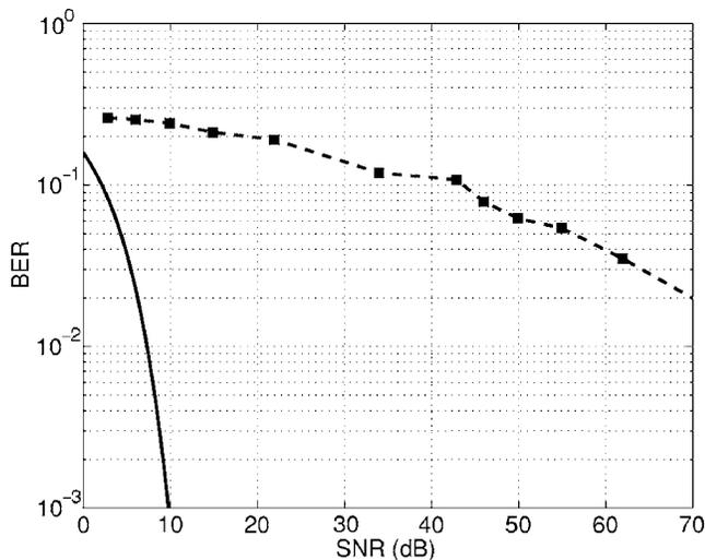
FIG. 12. Probability of bit error (BER) as a function of the signal-to-noise ratio (SNR) for the proposed communication scheme. For comparison the case of a bipolar baseband signal (with matched filter) is shown (solid line).
