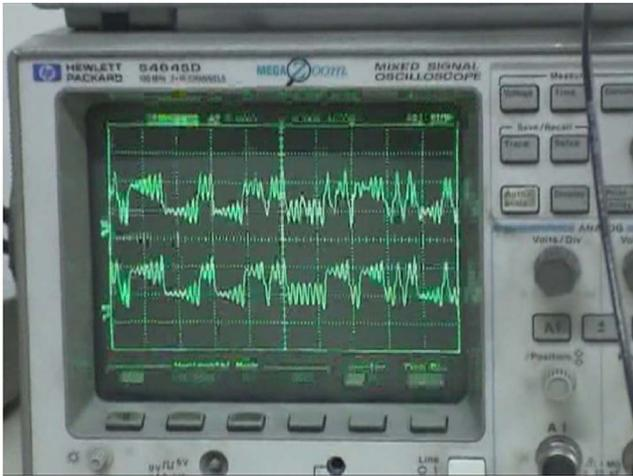
FIG. 9. (Color online) Trends of  $x_{2m}$  vs  $x_{2s}$  when the feedback is on. The two systems are synchronized except for some mismatches due to circuital parameter tolerances.
