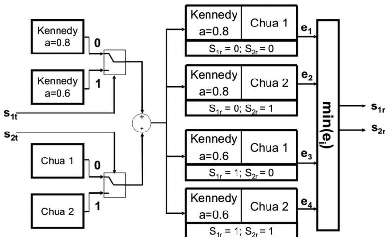
FIG. 10. Communication scheme based on the idea of separation and synchronization of chaotic signals.
