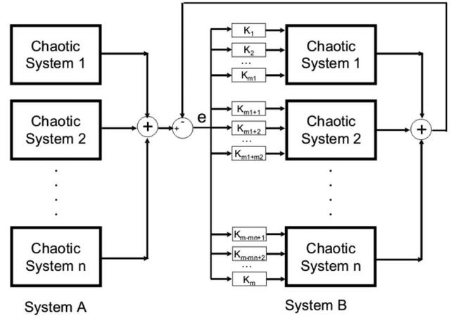
FIG. 1. Separation and synchronization scheme. 1-1', 2-2', and  $n$ - $n'$  are identical systems starting from different initial conditions; the error is the difference between a linear combination of the state variables of the master system and those of the slave system.
