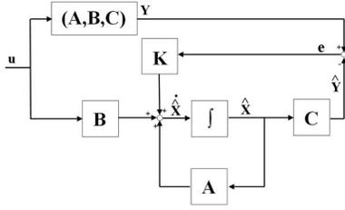
FIG. 2. Block scheme of a generic asymptotic linear observer.  $(A, B, C)$  are the system state matrices,  $K$  is the observer gains vector.
