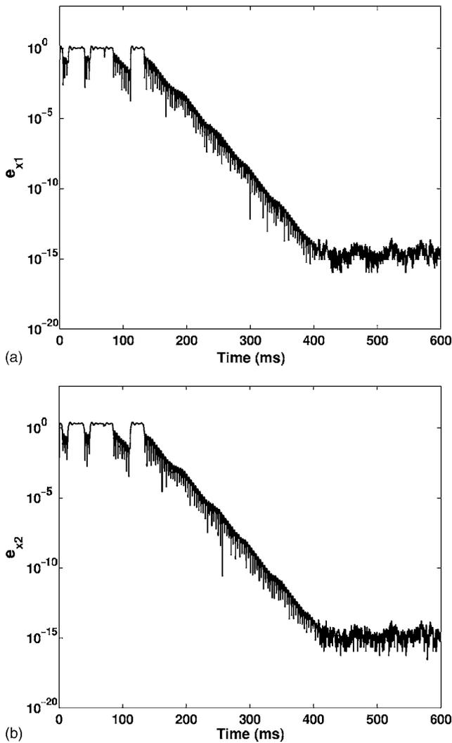
FIG. 7. Separation and synchronization of a pair composed by a Chua's circuit and a Kennedy's oscillator. Semilogarithmic plot of the absolute error for (a)  $x_1$  and (b)  $x_2$ .
