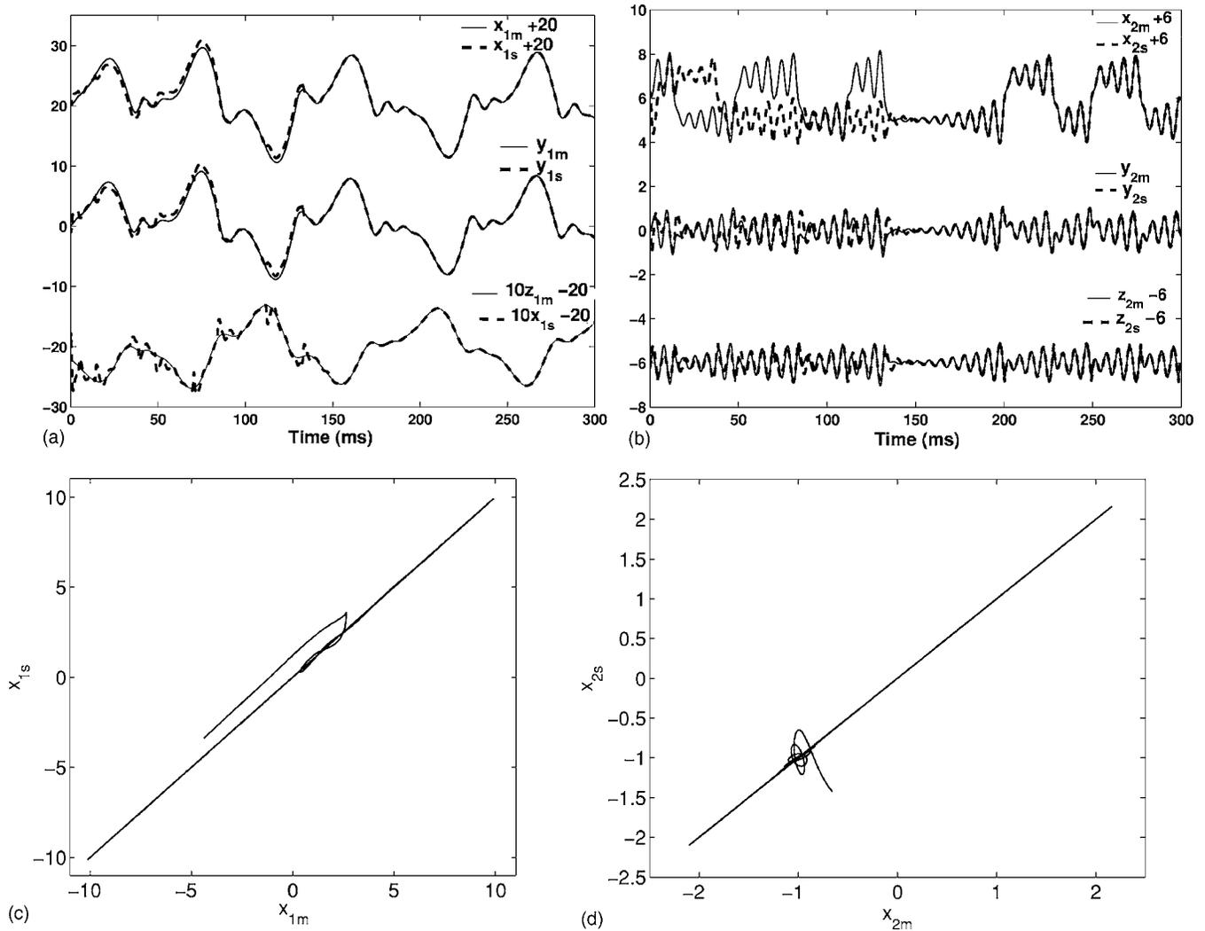
FIG. 6. Separation and synchronization of a pair composed by a Chua's circuit and a Kennedy's oscillator. (a) Trend of  $x_{1m}+20$ ,  $y_{1m}$  and  $z_{1m}-20$  (continuous lines) compared to  $x_{1s}+20$ ,  $y_{1s}$  and  $z_{1s}-20$  (dotted lines), (b) trend of  $x_{2m}+6$ ,  $y_{2m}$  and  $z_{2m}-6$  (continuous lines) compared to  $x_{2s}+6$ ,  $y_{2s}$  and  $z_{2s}-6$  (dotted lines), (c) synchronization plot  $x_{1m}$  vs  $x_{1s}$ , (d) synchronization plot  $x_{2m}$  vs  $x_{2s}$ .
