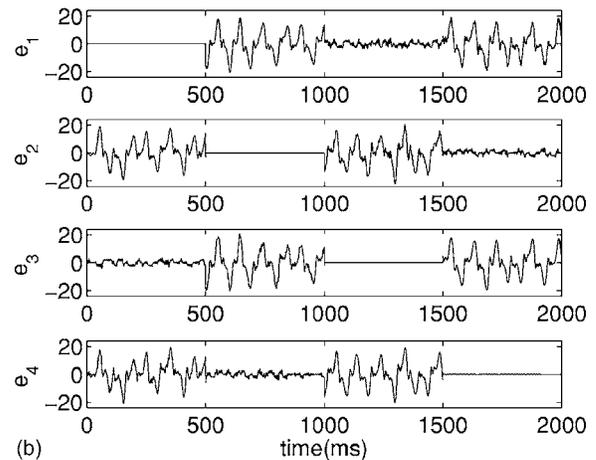
FIG. 11. (a)  $S_{1t}$  and  $S_{2t}$  are the transmitted information masked in the two different chaotic signals, while  $S_{1r}$  and  $S_{2r}$  are the detected signals using the separation and synchronization transmission scheme shown in Fig. 10. (b)  $e_1$ ,  $e_2$ ,  $e_3$ , and  $e_4$  are the synchronization errors of the four slave systems  $C_1$ ,  $C_2$ ,  $C_3$ , and  $C_4$ .
