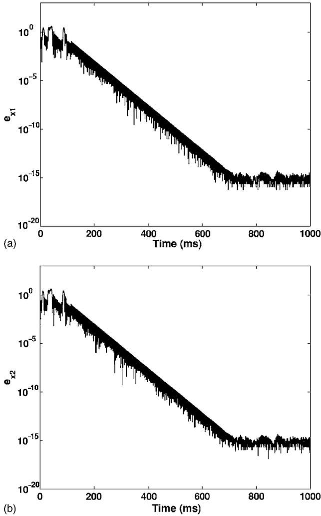
FIG. 4. Separation and synchronization of two Kennedy's oscillators. Semilogarithmic plot of the absolute error for (a)  $x_1$  and (b)  $x_2$ .
