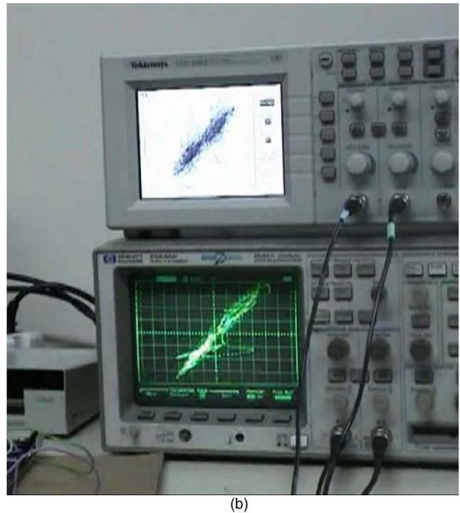
FIG. 8. (Color online) Separation and synchronization of a pair of Kennedy's oscillators. Synchronization plot,  $x_{1m}$  vs  $x_{1s}$  on the upper oscilloscope,  $x_{2m}$  vs  $x_{2s}$  on the lower oscilloscope. (a) Without feedback, there is no synchronization. (b) With feedback, separation and synchronization are achieved.
