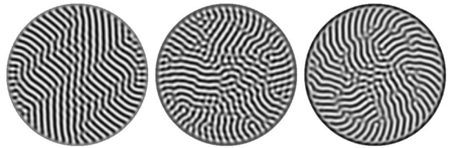
FIG. 3. Simulation of the Boussinesq equations with \Gamma=20 , \sigma=0.93 , \Omega=17.6 , \varepsilon=0.055 , and an artificially large centrifugal force in order to model the effect of an inaccessible large \Gamma . Left: zero centrifugal force. Center: centrifugal force is four times the physical value. Right: centrifugal force is ten times the physical value. A movie of this sample at 100 \times actual speed is available [30].
