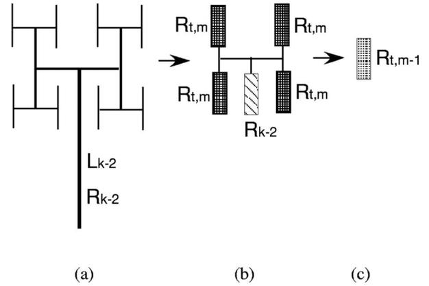
FIG. 3. (a) The  $(k-1)$  level network, (b) the corresponding thermal resistance network, and (c) the total effective resistance of the network.
