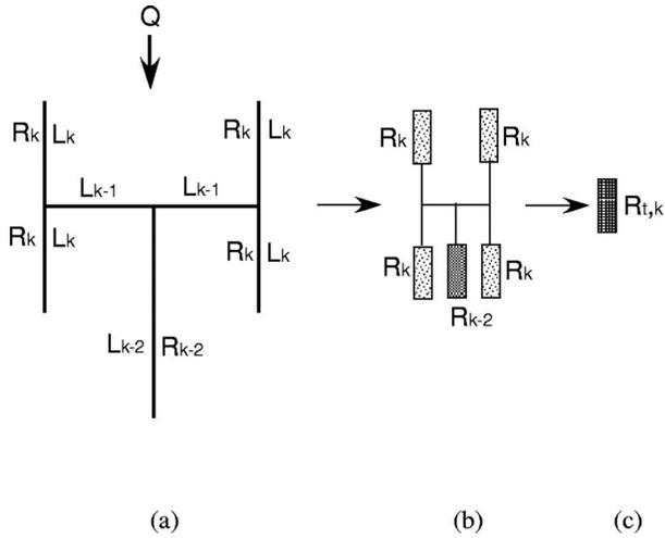
FIG. 2. (a) The  $k$ th level network, (b) the corresponding thermal resistance network, and (c) the total effective resistance of the network.
