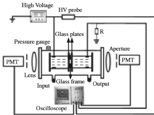
FIG. 2. Schematic diagram of the experimental setup.
