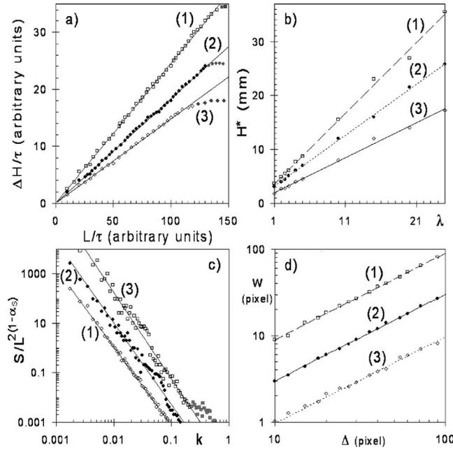
FIG. 2. (a) Data collapse for sheet heights  $\Delta H(L, \tau)$  and (b) graphs of the sheet roughness amplitude,  $H^*$ , vs scaling factor of sheet size  $\lambda$ ; (c) Data collapse for size dependent structure factor (3) of sheet profiles (in arbitrary units) and (d) Log-log graphs of local profile roughness  $w(\Delta)$  vs window size  $\Delta$  for Filtro papers with closed (1), medium (2), and open (3) porosity.
