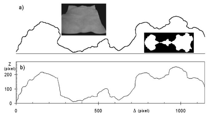
FIG. 1. (a) Profile of crumpled Filtro paper with closed porosity (inserts show photograph of crumpled sheet (top) and the closed contour profile presentation (bottom) used for perimeter-area measurements) and (b) its digitized single-valued presentation.
