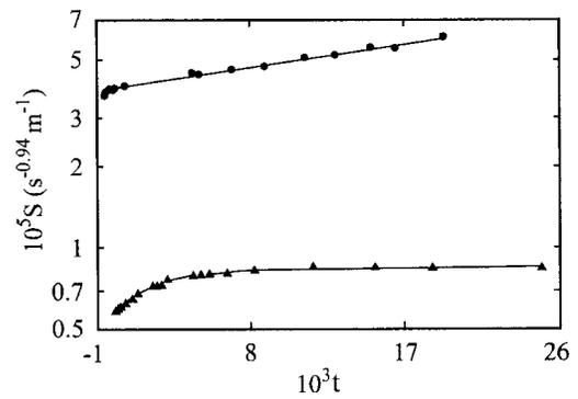
FIG. 4. Amplitude  $S$  of the Bhattacharjee-Ferrell theoretical model [Eq. (19)] as a function of reduced temperature  $t$  for the  $i\text{-C}_4\text{E}_1\text{-H}_2\text{O}$  ( $\bullet$ ) and the nitroethane-cyclohexane ( $\blacktriangle$ ) mixtures of critical composition. The lines are drawn to guide the eyes.
