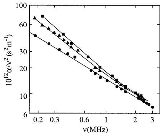
FIG. 2. Low-frequency part of frequency normalized acoustical attenuation spectra for the  $i$ -C<sub>4</sub>E<sub>1</sub>-H<sub>2</sub>O mixture of critical composition. •: 20.2 °C; ▲: 23.64 °C; ■: 24.95 °C.
