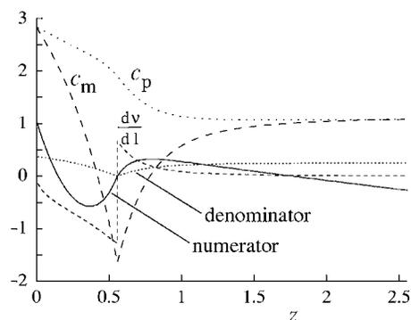
FIG. 3. The principal curvatures  $c_p$  and  $c_m$ , the derivative of the inclusion density  $d\nu/dl$ , and the numerator and denominator of the expression for  $d\chi/dl$  [Eq. (21)] for the critical shape whose parameters correspond to the shape (c) in Fig. 2.
