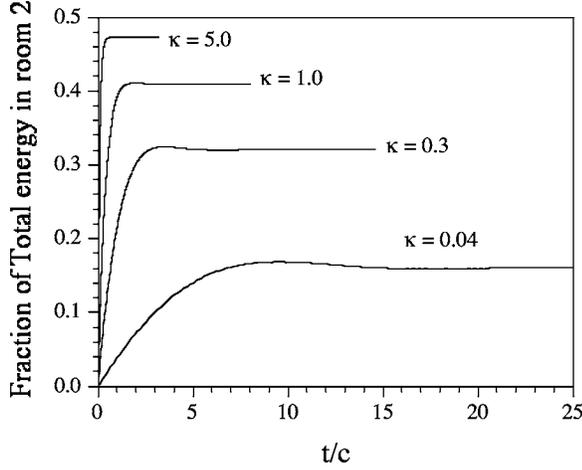
FIG. 2. Flow dynamics between two equal-sized rooms at various values of dimensionless coupling  $\kappa$ . Time is in units of modal density  $c$ .
