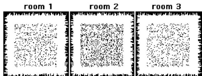
FIG. 6. The three-room structure. The points represent randomly positioned springs coupling adjacent rooms.
