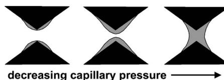
FIG. 4. Schematic of snapoff in a pore throat. Black denotes pore-throat wall, gray water, and white gas.
