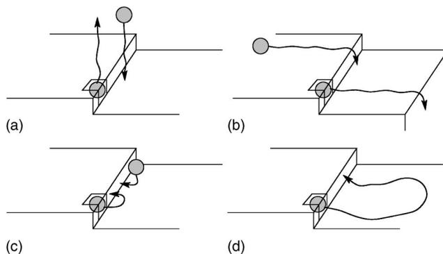
FIG. 1. Different types of step dynamics with (a) and (b) being type I (nonconserving and uncorrelated); (c) being type II (local conserving); and (d) being type III (nonlocal conserving). The shaded circles depict adatoms.
