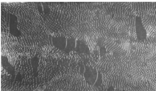
FIG. 9. Picture of the same foam as in Fig. 8, taken few seconds later, 50 cm downstream in the cell. The foam flow is oriented to the right. Some of the ten large bubbles have spontaneously organized in a few bubble columns oriented along the flow. A few bubbles of intermediate size are due to a few undesirable film breakages and are disregarded.
