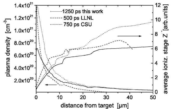
FIG. 8. Dependence of the plasma density and average ionization stage on the distance from the target surface at the time of optimum delay. The simulation was performed with the prepulse parameters of the reported experiments at Max-Born-Institute (MBI,  $1 \times 10^{11}$  W/cm<sup>2</sup>, 400 ps), Colorado State University [7] (CSU,  $2.4 \times 10^{12}$  W/cm<sup>2</sup>, 120 ps), and Lawrence Livermore National Lab [2] (LLNL,  $5 \times 10^{11}$  W/cm<sup>2</sup>, 200 ps).
