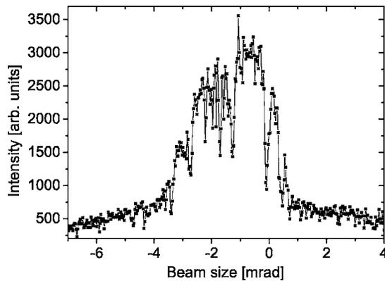
FIG. 6. Lineout of the image of lasing traced along the recorded line to determine the XRL beam divergence. The dips in the shape are caused by the supporting structure of the Al filter foil. For the pump pulse parameters, see Fig. 7(a).
