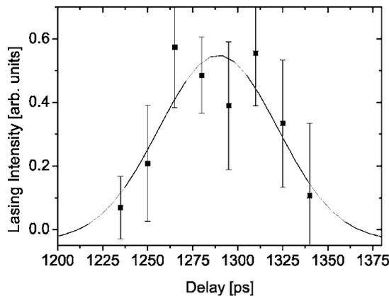
FIG. 3. Dependence of the x-ray laser output signal on the delay between both pump pulses. Each measurement point is a result of averaging over 10 shots. Parameters as in Fig. 4.
