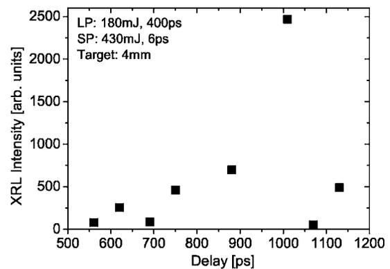
FIG. 5. Delay temporal window for lasing achieved with more energetic pumping. The best results for each delay setting are shown.
