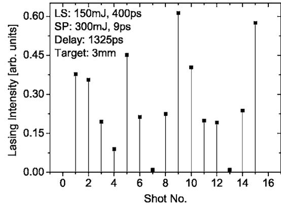
FIG. 4. Sequence of XRL pulses registered with a repetition rate of about 1 Hz.
