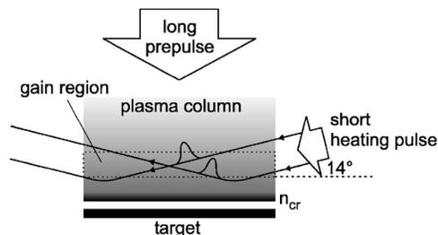
FIG. 1. Sketch explaining the GRIP principle and double irradiation of the active area by the pump beam.
