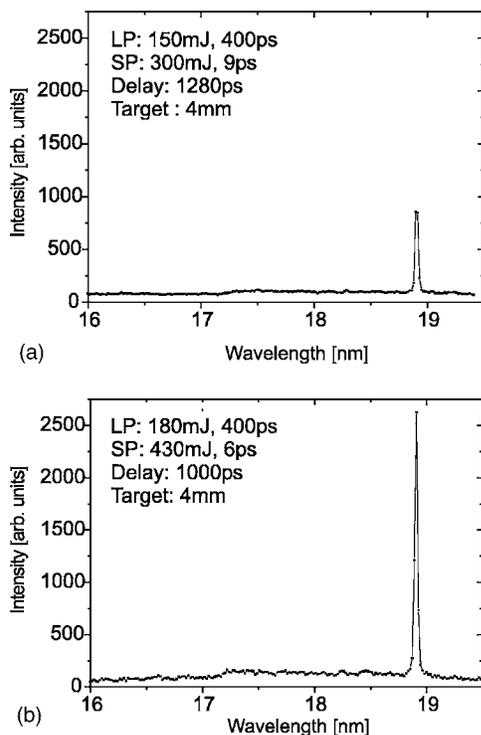
FIG. 7. Soft x-ray spectrum with dominating Ni-like Mo lasing line at 18.9 nm. The step in the spectrum at around 17.2 nm is caused by the absorption  $L$  edge of Al used as a filter.
