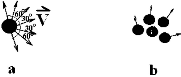
FIG. 3. (a) If a collision occurs, a pedestrian chooses one of the possible velocity, and detect whether the path of chosen direction is passable. (b) There is no way to go and the pedestrian has to stop.
