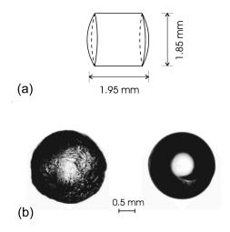
FIG. 2. (a) A diagram of the pasta grains and (b) two photographs of the glass beads before (right) and after (left) the treatment with fluorhidric acid (series 2 and 5, respectively).
