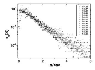
FIG. 5. Histogram for the number of grains of the avalanches normalized with the mean avalanche size  $\langle s \rangle$ . Different symbols correspond to 14 histograms from R=1.52 to R=3.96 that are plotted together. It can be seen that all the histograms collapse into a single curve.
