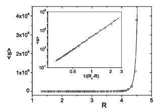
FIG. 6. Mean avalanche size  $\langle s \rangle$  vs R. The symbols  $\square$  represent experimental points obtained from the histograms. The solid line is the fit with Eq. (1). Inset: mean avalanche size  $\langle s \rangle$  vs  $1/(R_c - R)$ . Note the logarithmic scale.
