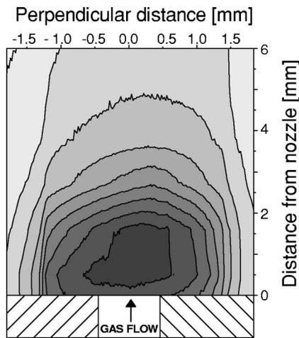
FIG. 2. Time-integrated contour map of the total plasma emission. Also indicated is a section of the nozzle, showing the 1-mm-diameter opening for gas flow. The various contours correspond to changes in steps of 10% in emission, or  $\sim 3\%$  in density. The laser was incident from the left and focused at a distance of  $160 \mu\text{m}$  from the nozzle surface. The views for the present spectroscopic measurements were centered at distances of  $1.6 \pm 0.5$  and  $6.0 \pm 0.5$  mm.
