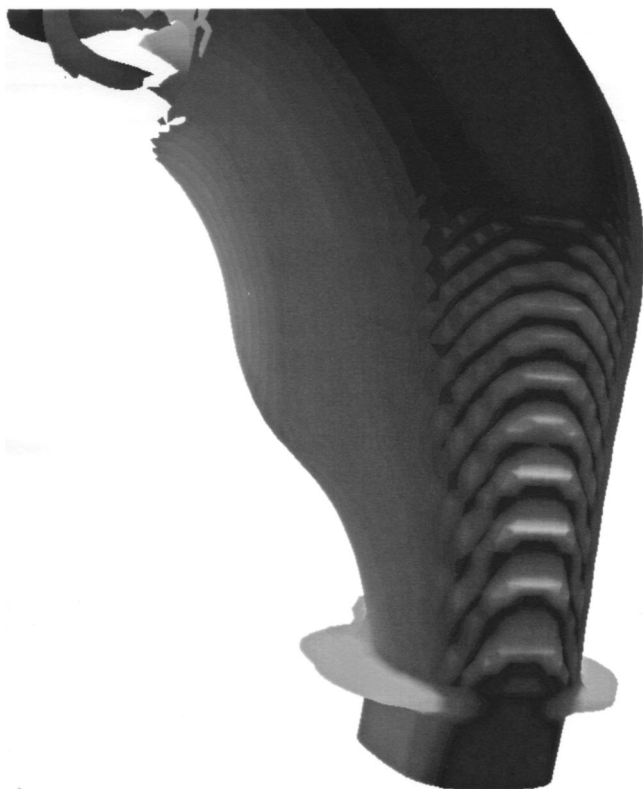
FIG. 6. Development of Kelvin-Helmholtz rollers for the velocity ratio R=3.5 as revealed by contours of \omega_y vortices. t=9 , Re=225 .
