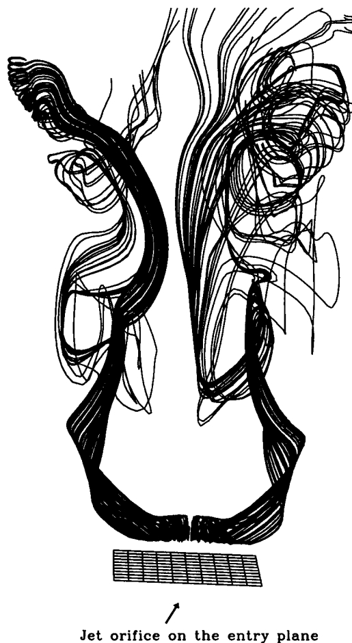
FIG. 7. Three-dimensional evolution of streamlines participating in the formation of a Kelvin-Helmholtz vortex at t=21.0 . Re=225 , R=2.5 .
