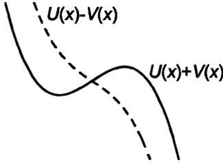
FIG. 1. Switching potential with metastable state.
