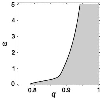
FIG. 3. Shaded area is the parameter region on the plane  $(q, \omega)$  where NES effect can be observed. Here  $\omega = (\nu L)/k$ ,  $q = a/k$ , and  $b = 2L$ .
