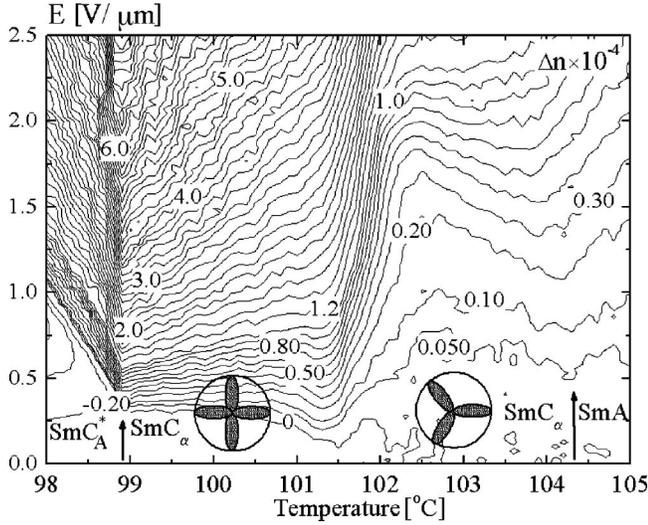
FIG. 3.  $E$ - $T$  phase diagram of the field-induced birefringence in a 25- $\mu\text{m}$ -thick homeotropic cell of (S)-MHPOCBC. The labels of constant birefringence correspond to values  $\Delta n \times 10^{-4}$ .
