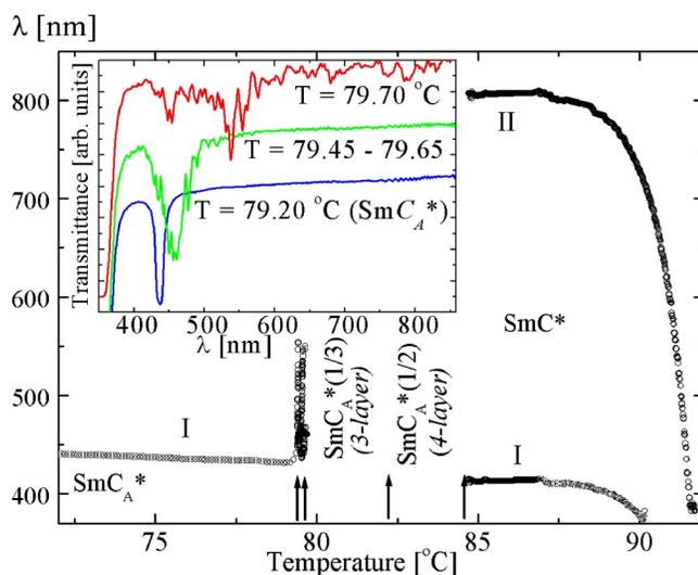
FIG. 2. (Color online) Characteristic reflection peaks for 20° oblique incidence in a 60- $\mu\text{m}$ -thick free-standing film of (R)-12OF1M7. The inset illustrates typical characteristic reflection spectra at the indicated temperatures.
