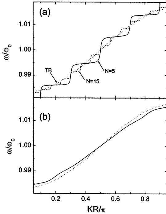
FIG. 3. (a) The  $\omega(k)$  dispersion curves of the CROW structures  $\text{air}/(\text{LHLHLHLHL})^N/\text{air}$ , where  $N$  is 5 (solid curve), 15 (dashed curve), and  $\infty$  (dotted curve), respectively. (b) The  $\omega(k)$  dispersion curves of the CROW structures  $\text{air}/\text{HLHL} \times (\text{LHLHLHLHL})^5\text{LHLH}/\text{air}$  (solid curve) and  $\text{air}/(\text{LHLHLHLHL})^\infty/\text{air}$  (dotted curve), respectively.
