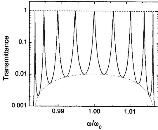
FIG. 5. The transmission spectrum (solid curve) and  $T_{\min}(\lambda)$  curve (dotted curve) of the CROW air/(LHLHLHLHL)<sup>10</sup>/air. The straight dashed line is the unity transmittance.
