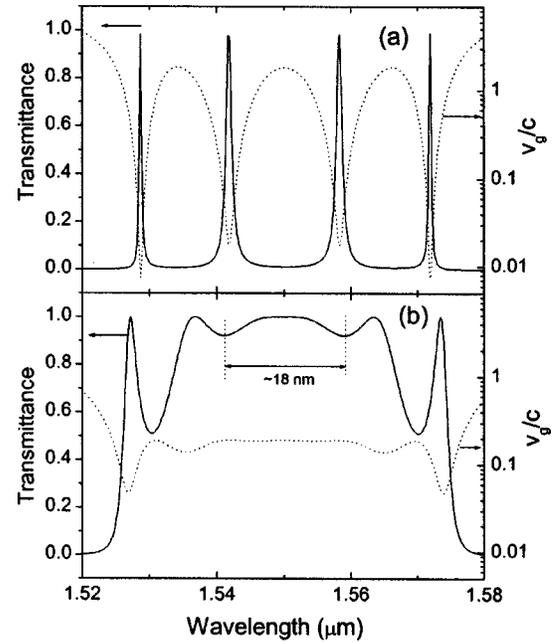
FIG. 2. (a) The enlarged view of the transmission (solid curve) and group velocity (dotted curve) curves around the central wavelength of the CROW structure  $\text{air}/(\text{LHLHLHLHL})^5/\text{air}$ . (b) The transmission (solid curve) and group velocity (dotted curve) curves of the CROW structure  $\text{air}/\text{HLHL}(\text{LHLHLHLHL})^5\text{LHLH}/\text{air}$ .
