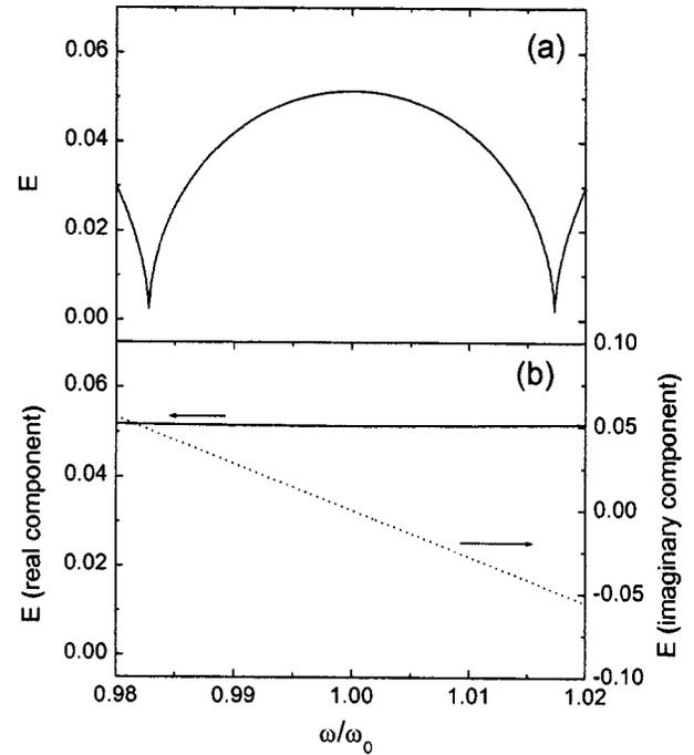
FIG. 4. (a) The equivalent admittance of the unit cell  $\text{LHLHLHLHL}$ . (b) The real component (solid curve) and the imaginary component (dot curve) of equivalent admittance of the matching layer stack  $\text{air}/\text{HLHL}$ .
