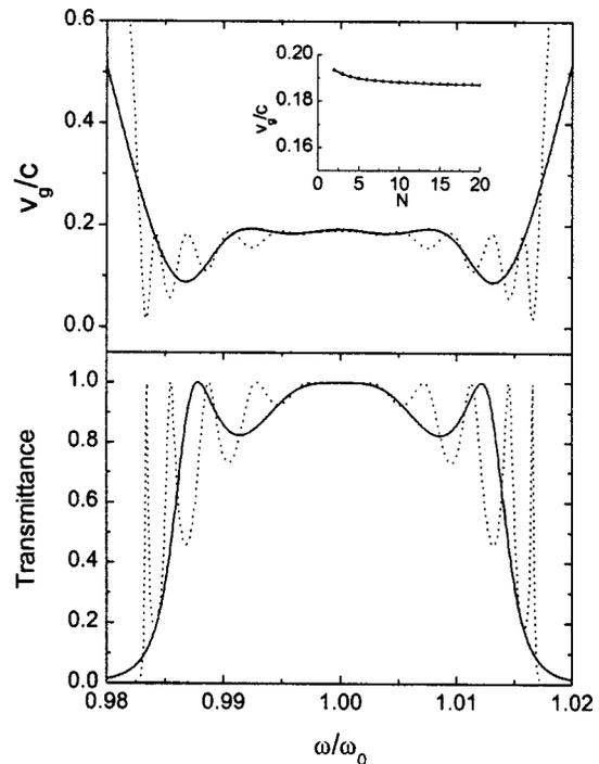
FIG. 7. The group velocity and the transmittance curves of the CROW  $\text{air}/HLHL (LHLHLHLHL)^N LHLH/\text{air}$  with  $N=3$  (solid curve) and 10 (dotted curve). The inset shows  $v_g(\lambda_0)$  versus the number of unit cell  $N$ .
