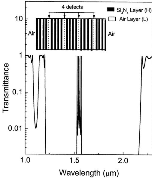
FIG. 1. The transmission spectrum of the CROW structure  $\text{air}/(\text{LHLHLHLHL})^5/\text{air}$  calculated by the  $T$ -matrix method, where  $H(L)$  represents the quarter-wave  $\text{Si}_3\text{N}_4$  (air) layer. The inset shows the schematic sketch of the CROW  $\text{air}/(\text{LHLHLHLHL})^5/\text{air}$ .
