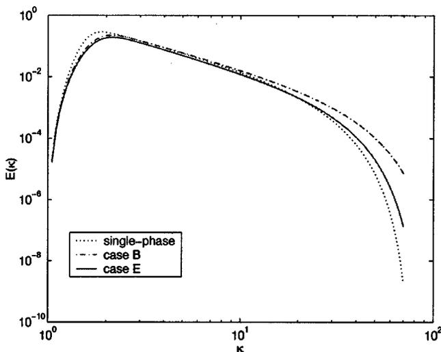
FIG. 8. Dimensionless turbulent kinetic energy of the carrier fluid as a function of dimensionless wave number ( $\tau \approx 1.5$ ).
