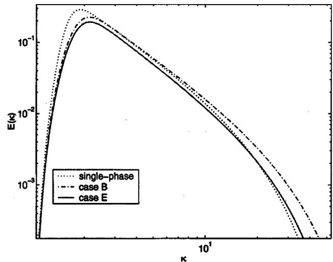
FIG. 9. Dimensionless turbulent kinetic energy of the carrier fluid as a function of dimensionless wave number ( $\tau \approx 1.5$ ). (Enlargement of Fig. 8.)
