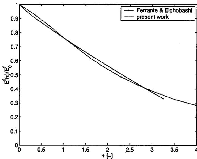
FIG. 3. Dimensionless turbulent kinetic energy of the fluid as function of dimensionless time for the particle-free case. Comparison between model predictions and DNS results.
