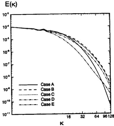
FIG. 2. Dimensionless kinetic energy of the carrier fluid as function of dimensionless wave number at  $t=5.0$ . From Ferrante and Elghobashi [9].
