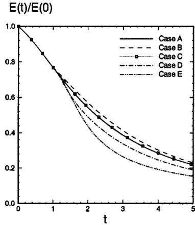
FIG. 1. Dimensionless turbulent kinetic energy as a function of dimensionless time. From Ferrante and Elghobashi [9].
