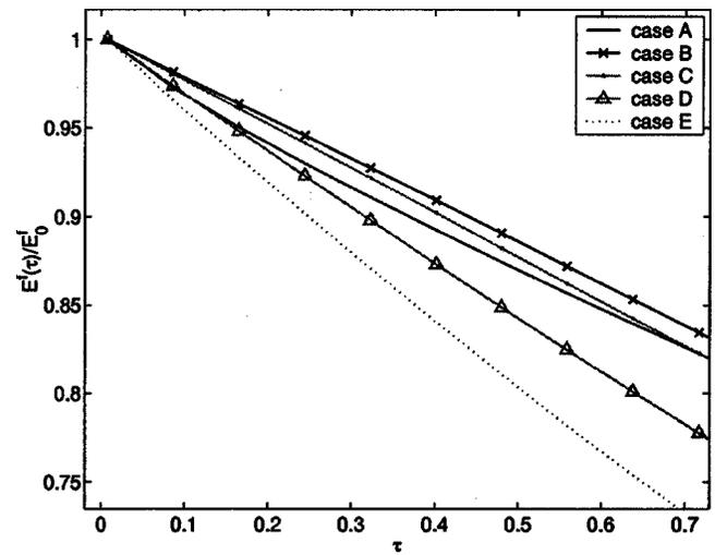
FIG. 5. Dimensionless turbulent kinetic energy of the carrier fluid in a suspension as a function of dimensionless time ( $0 < \tau < 0.7$ ).
