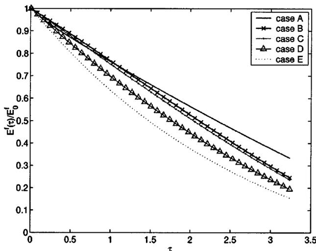
FIG. 4. Dimensionless turbulent kinetic energy of the carrier fluid in a suspension as a function of dimensionless time ( $0 < \tau < 3.5$ ).
