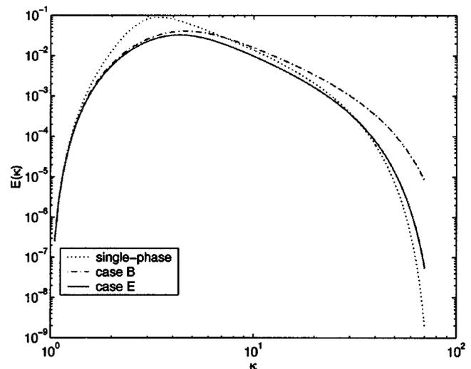
FIG. 10. Dimensionless turbulent kinetic energy of the carrier fluid as a function of dimensionless wave number ( $\tau \approx 3.0$ ).
