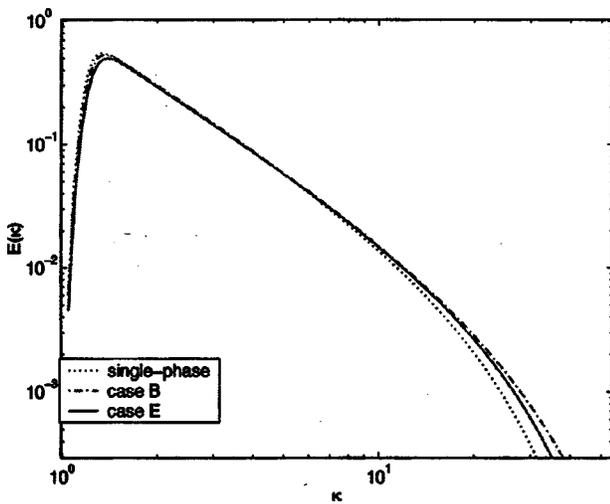
FIG. 7. Dimensionless turbulent kinetic energy of the carrier fluid as a function of dimensionless wave number ( $\tau \approx 0.5$ ). (Enlargement of Fig. 6.)
