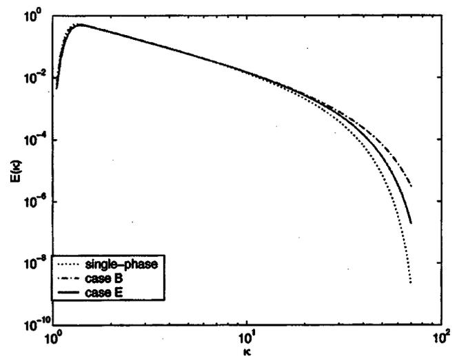
FIG. 6. Dimensionless turbulent kinetic energy of the carrier fluid as a function of dimensionless wave number ( $\tau \approx 0.5$ ).
