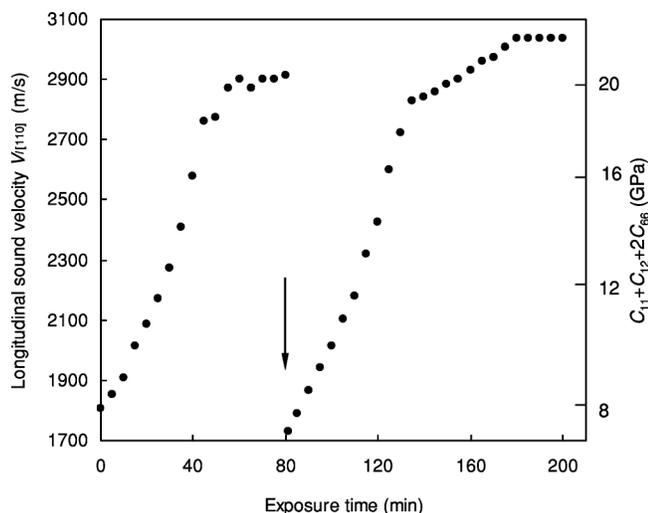
FIG. 2. Reversible change in longitudinal sound velocity  $V_{[110]}$  along [110] direction in a tetragonal HEW lysozyme crystal as a function of exposure time to open air. The time, at which the dried crystal was immersed in solution, is indicated by an arrow.
