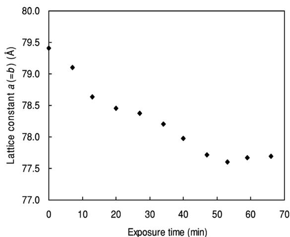
FIG. 4. Change in lattice parameters  $a (=b)$  of a tetragonal HEW lysozyme crystal as a function of exposure time to open air.
