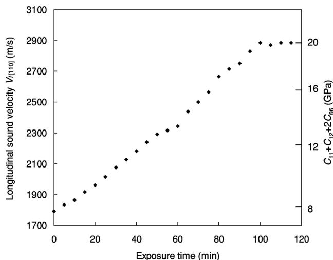
FIG. 1. Change in longitudinal sound velocity  $V_{[110]}$  along [110] direction in a tetragonal HEW lysozyme crystal as a function of exposure time to open air. The scale of composite elastic constant,  $C_{11}+C_{12}+2C_{66}$ , corresponding to the longitudinal sound velocity  $V_{[110]}$  is denoted as ordinate on right in the figure.
