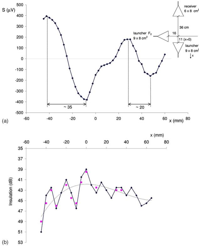
FIG. 2. (a) Same as Fig. 1, with  $F_1$  and  $F_2$  in vp and no attenuation, as function of the position ( $x$  coordinate in the inset) of the launcher  $F_1$ ; (b) measured insulation between the horns having  $F_2$  as launcher and  $F_1$  as receiver. The continuous line represents an “average” of the data.
