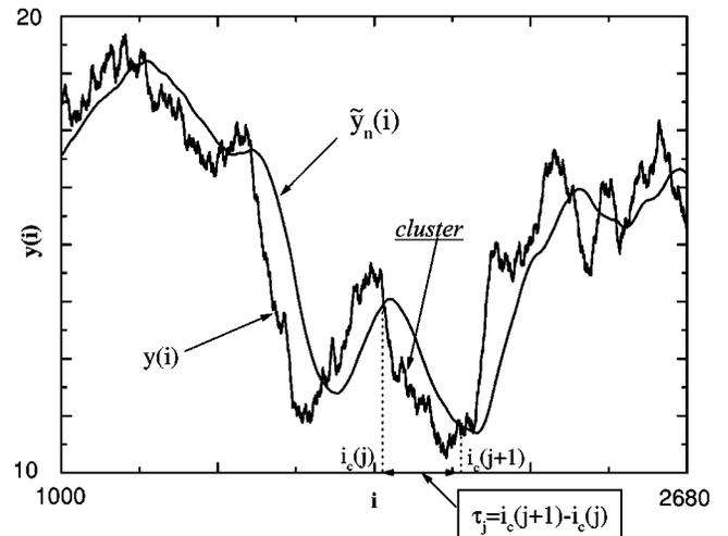
FIG. 1. Stochastic series  $y(i)$  of length  $N_{\max} = 2^{19}$  obtained by the random midpoint displacement algorithm with  $H = 0.8$ . Also shown is the moving average  $\bar{y}_n(i)$ , with box dimension  $n = 30$ . The time interval between two subsequent crossing points  $y(i)$  and  $\bar{y}_n(i)$  define the length  $\ell_j$ , the duration  $\tau_j$ , and the area  $s_j$  of the cluster according to Eqs. (5), (6), and (7).
