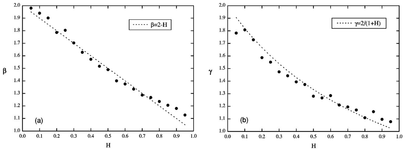
FIG. 5. (a) The exponent  $\beta$  vs  $H$  [Eq. (10)] for series having different  $H$  ( $H=0.05-0.95$  with step size  $0.05$ ). The relationship  $\beta = 2 - H$  is also shown (dashed line). (b) Plot of the exponent  $\gamma$  vs  $H$  [Eq. (15)] for series having different  $H$  ( $H=0.05-0.95$  with step  $0.05$ ). The relationship  $\gamma = 2/(1 + H)$  is also shown (dashed line).
