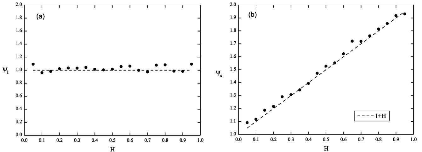
FIG. 3. Plot of the exponents (a)  $\psi_\ell$  vs  $H$  [Eq. (8)] and (b)  $\psi_s$  vs  $H$  [Eq. (9)] for series having different  $H$  [from  $H=0.05$  to  $0.95$  in steps of size  $0.05$  (circles)]. The relationships  $\psi_\ell=1$  and  $\psi_s=1+H$  are shown (dashed lines).
