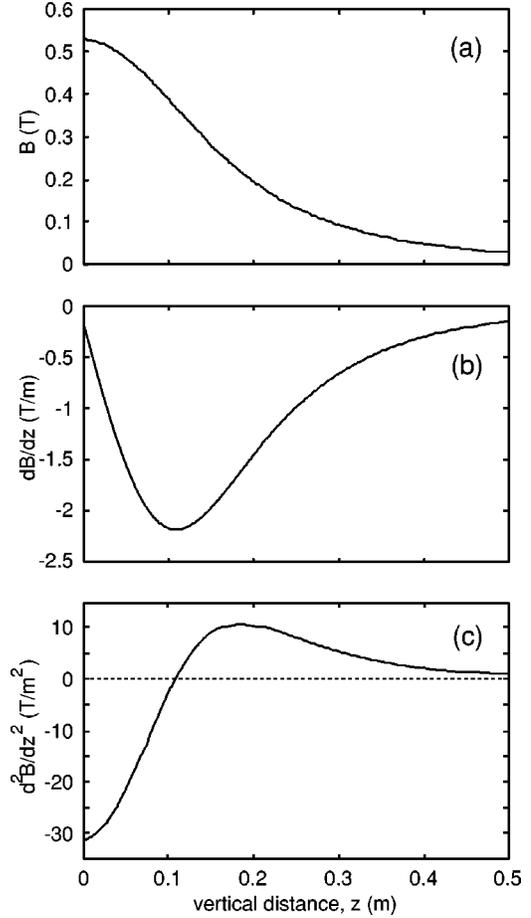
FIG. 2. Magnetic field on the axis of the magnetic coils at the current of 1 kA. (a) Magnetic induction, (b) first and (c) second spatial derivatives. The field is produced by a 17 cm thick coil with 30 cm bore. The current can be varied from 0 to 1.6 kA.
