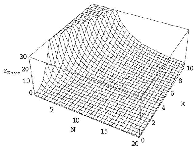
FIG. 3. Variation of site-specific association rate ( $r_{Kave}$ ,  $\text{mol}^{-1} \text{s}^{-1}$ ) with respect to changes in DNA length ( $N$  in base pairs) and jump size ( $k$ , in base pairs) (when  $N$  and  $k$  are independent quantities), which clearly shows a constant nature of  $r_{Kave}$  at higher  $N$  and  $k$ .
