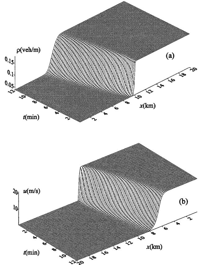
FIG. 1. Shock waves under the Riemann initial conditions of Eq. (22a): temporal evolution of (a) density  $\rho(x,t)$  and (b) velocity  $u(x,t)$ .
