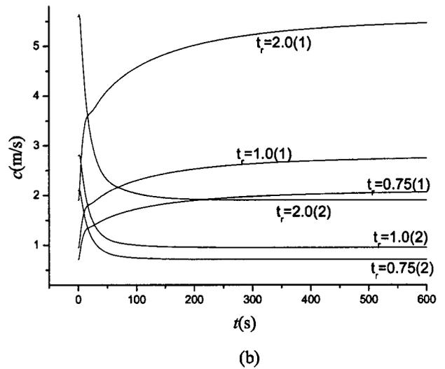
FIG. 3. The variation of propagation velocity  $c(\rho)$  of a disturbance of vehicle density and its temporal evolution under the two Riemann initial conditions of Eqs. (22a) and (22b), respectively labeled as (1) and (2).
