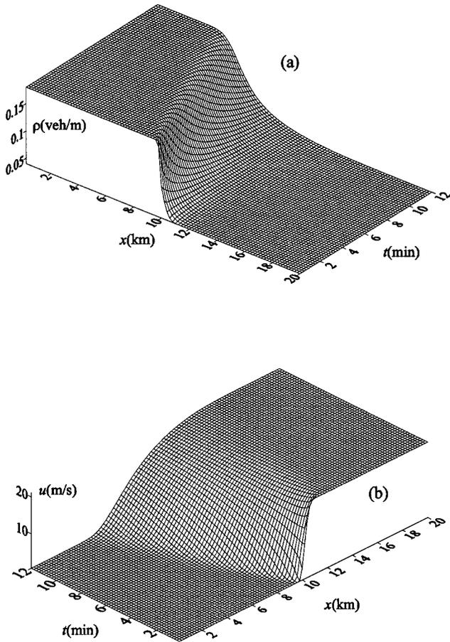
FIG. 2. Rarefaction waves under the Riemann initial conditions of Eq. (22b): temporal evolution of density  $\rho(x,t)$  and (b) velocity  $u(x,t)$ .
