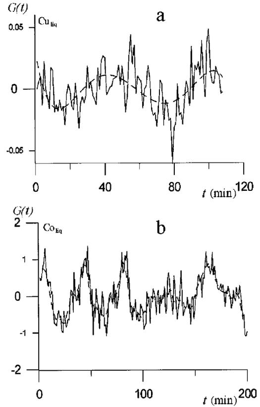
FIG. 3. Time dependences of autocorrelation function for liquid copper (a) and liquid cobalt (b) viscosity close to corresponding temperatures of step change of viscosity.
