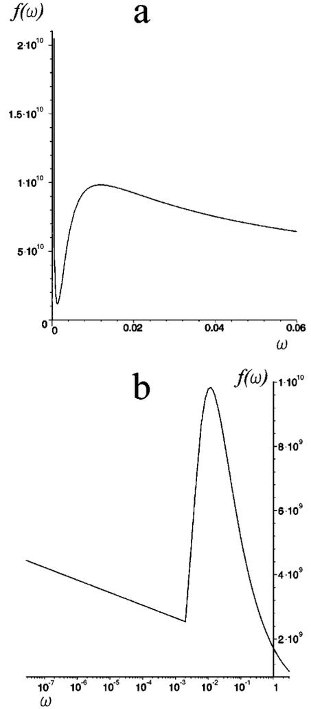
FIG. 6. The spectrum of viscosity oscillations [ $f(\omega) = \sqrt{f_1(\omega)^2 + f_2(\omega)^2}$ ] in linear-linear (a) and logarithmic-linear (b) coordinates.
