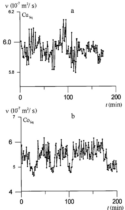
FIG. 1. Time dependences of kinematic viscosity of liquid copper [9,10] (a) and liquid cobalt (1870 K) [8] (b) close to the temperature of step change of viscosity.
