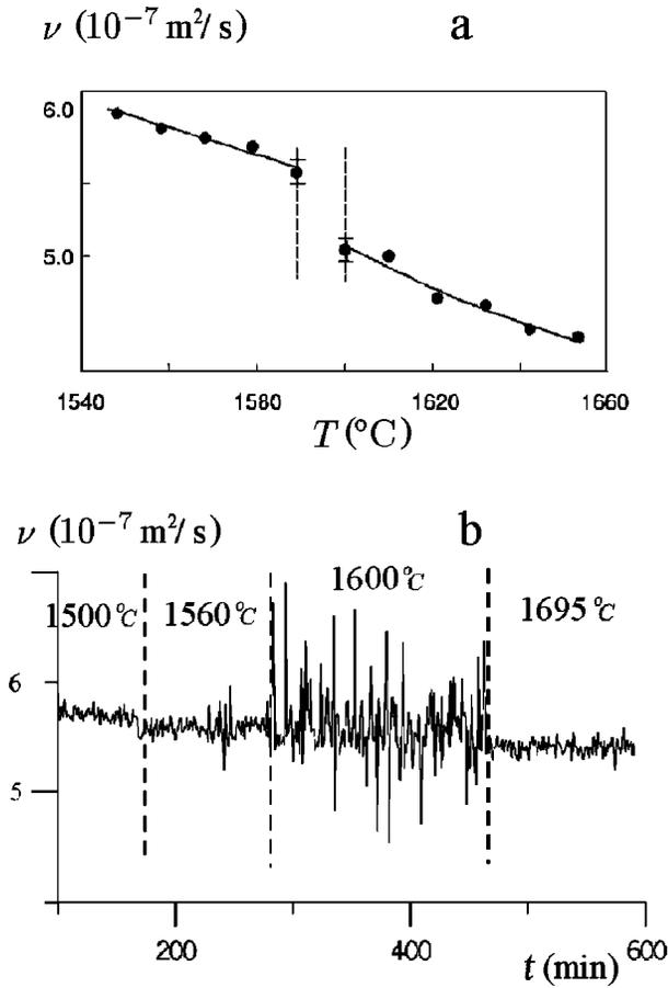
FIG. 2. Temperature dependence of kinematic viscosity of liquid cobalt (a) and time dependence of liquid cobalt viscosity at various temperatures (b).
