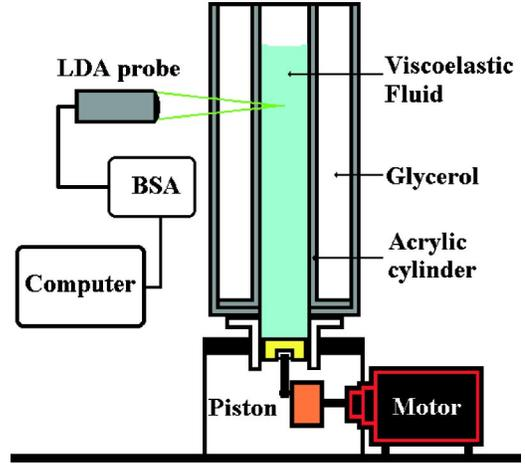
FIG. 1. Schematic view of the setup used for the study of the dynamic response with a LDA measuring system.
