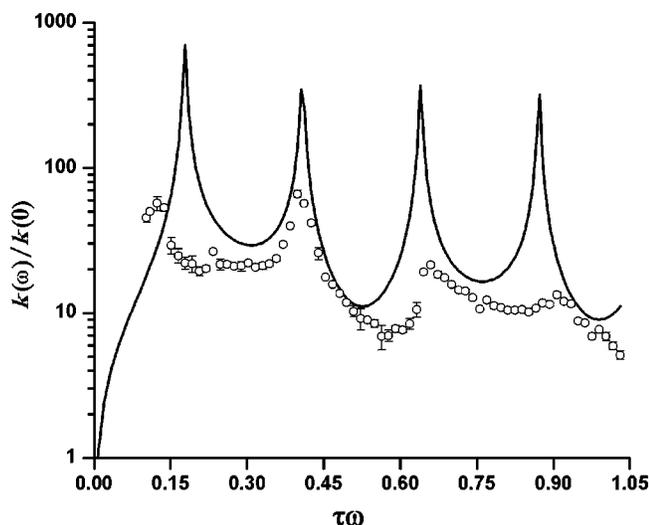
FIG. 4. Dynamic response for the CPyCl/NaSal solution. Experimental values are shown by circles [Eq. (9)] and the line represents the theoretical prediction [magnitude of  $\xi$  from Eq. (7)].
