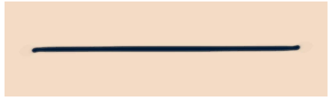
FIG. 1. For zero Reynolds number a two-dimensional droplet remains hydrodynamically stable at all \text{Ca} studied. It extends until the width of the droplet is of the order of the interface width. The picture shows a droplet with \text{Ca} = 1.1 ; the upper wall is moving rightward, the lower, leftward.
