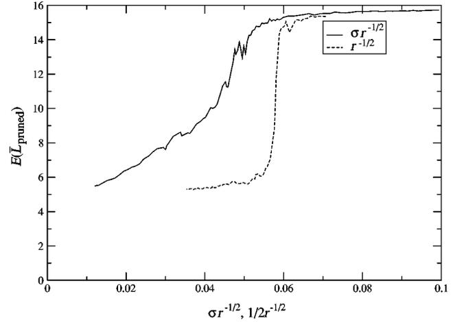
FIG. 7. The expected pruned tour length for annealings when  $r$  and  $1/T = \sqrt{r}/\sigma$  are increased monotonically. The sharp drop in the pruned tour length is seen when only  $r$  is controlled, demonstrating that this “freeze in” imperfections in the tour. The system was annealed at each value of the temperature and value of  $r$  for 50 000 Monte Carlo steps with  $n=300$  and  $p=0.1$ .
