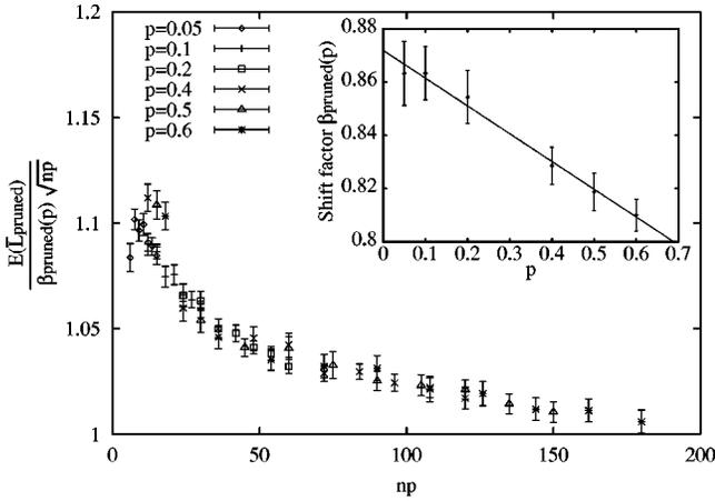
FIG. 3. The master curve for the pruned tour length divided by  $\beta_{\text{pruned}}(p)\sqrt{np}$ . The data follows a smooth curve for  $n > 30$ , and the shift factors follow a linear relationship, suggesting that  $E(\bar{L}_{\text{pruned}})/\sqrt{np}(0.872 - 0.105p) = f(np)$ . Three points with  $n = 30$  lie significantly above the other data points (here and also in Fig. 4), showing breakdown of the master curve at small  $n$ .
