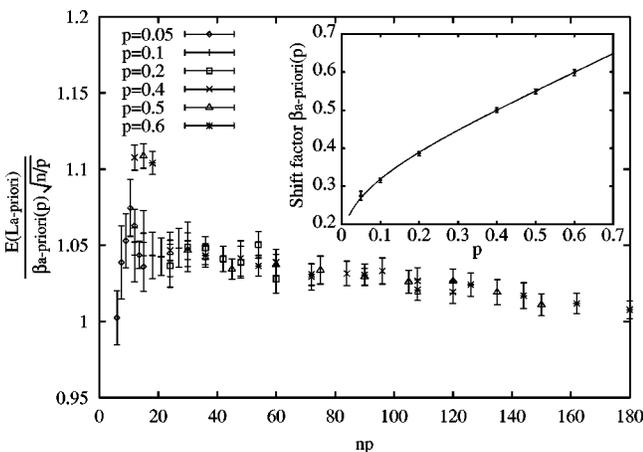
FIG. 4. The master curve for the *a priori* tour length divided by  $\sqrt{(n/p)}\beta_{a \text{ priori}}(p)$ . The shift factors, inset, are expected to tend towards a constant for  $p \rightarrow 0$ . The slight, but significant, deviation from linear suggests that this might not be the case.
