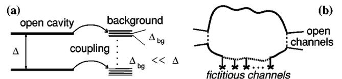
FIG. 1. An open cavity with absorption in walls modeled by coupling to (a) the compound background or (b) an infinite number of fictitious channels with vanishing transmission probabilities.
