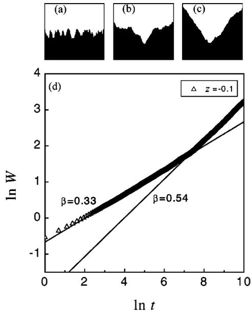
FIG. 4. (a)–(c) Typical time evolution of the surfaces for  $z = -0.5$  in a simulation sample. The used system size is  $L = 2^8$ . (a) The morphology at the initial stage of growth; (b) that around the time at which a valley bottom is formed; (c) that after the fully developed grooved is formed; (d) the time dependence of  $W$  in the early-time regime for  $z = -0.1$ .
