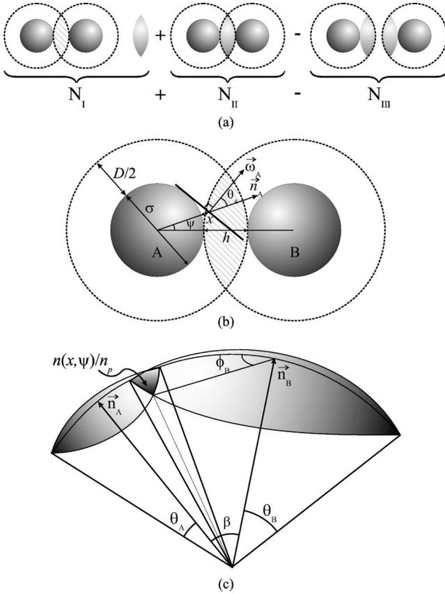
FIG. 4. (a) The three contributions to the excess adsorption density for  $h=D/2$ . (b) Definitions of the distances and angles of a disk in the overlapping depletion zone relative to sphere A. (c) The overlap of cones relative to spheres A and B [cf. Fig. 3(a)] determines the area accessible to a disk at a certain position between the two spheres.
