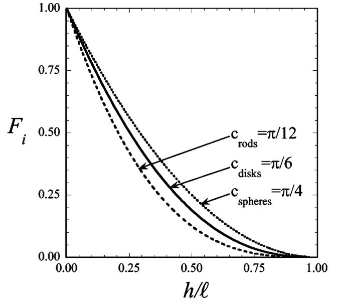
FIG. 2. The distance dependence  $F_i$  of the depletion potential of hard spheres due to the presence of other particles, Eq. (4), as a function of the scaled interparticle distance,  $h/\ell$ . The depth of the potential is given by  $c_i$ . Disks (full line,  $\ell = D$ ) are intermediate depletion agents compared to rods (dashed line,  $\ell = L$ ) and small spheres (dotted line,  $\ell = a$ ).
