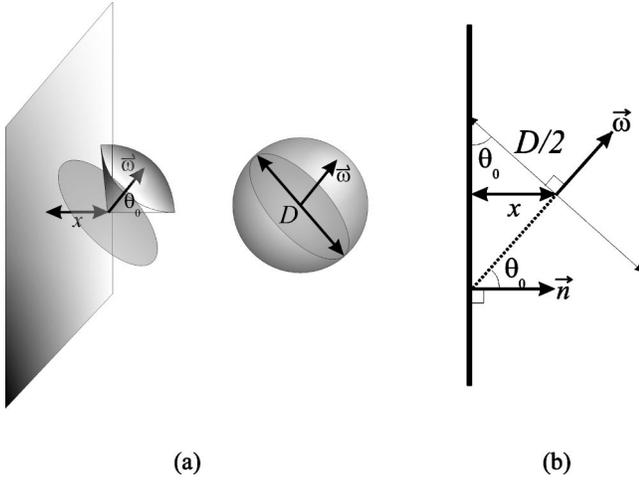
FIG. 3. (a) In the bulk the director  $\vec{w}$  of a disk with diameter  $D$  can describe a full unit sphere (right), whereas a disk at a distance  $x < D/2$  to a wall only describes part of it (left). (b) The maximum angle  $\theta_0$  between the director  $\vec{w}$  and the normal on a planar wall  $\vec{n}$  follows from  $\sin \theta_0 = x/(D/2)$ .
