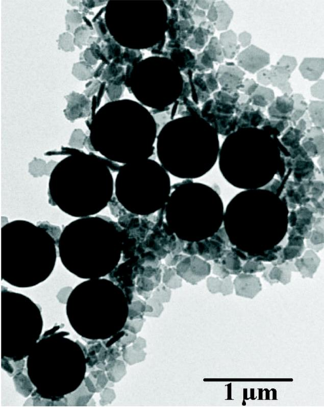
FIG. 1. TEM micrograph of a mixture of silica spheres ( $\sigma = 700$  nm) with silica coated gibbsite plates (diameter  $D = 200$  nm, thickness  $L = 30$  nm).
