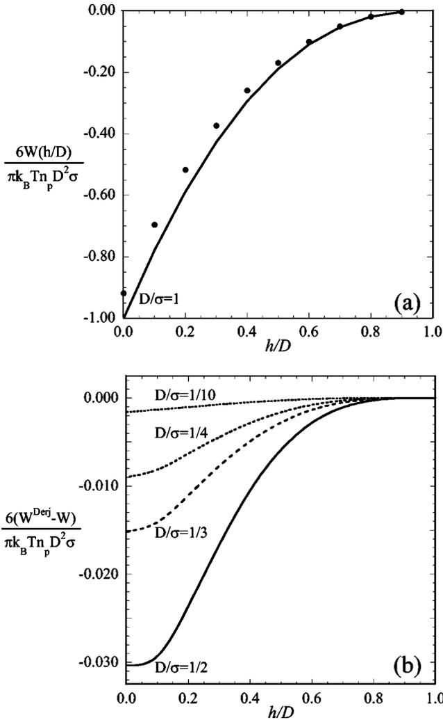
FIG. 5. (a) An actual profile (symbols) and Eq. (3) (solid line) for  $D/\sigma=1.0$ . (b) The difference of the distance dependence of the depletion potential of the exact solution compared to the Derjaguin approximation for several size ratios.
