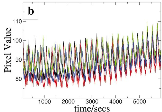
FIG. 4. (Color) Enhanced experimental image of in-phase synchronization (a), and the time series of the centers of the four cells (b). Initially they are out of phase, but eventually they synchronize in-phase.
