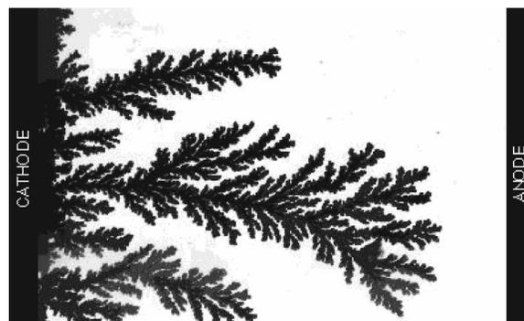
FIG. 1. Electrodeposition of copper on a glass substrate (reprinted with permission from Fleury). The quasi-two-dimensional cell is made of two copper electrodes and a  $\text{CuSO}_4$  solution (sample size  $3 \times 2 \text{ mm}^2$ ). Only a small part of the sample is shown.
