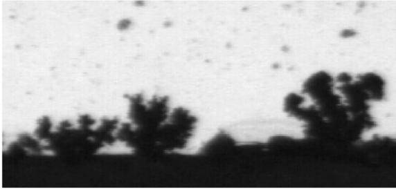
FIG. 2. Dendritic growth at the interface between a lithium electrode and a polymer electrolyte (courtesy Brissot [56]).
