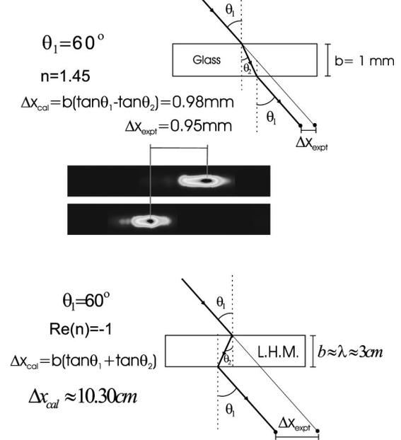
FIG. 3. Proposed experiment. Top panel: scheme for the experimental displacement measured in the streak camera with the parameters as indicated. Lower panel: the proposed experiment for a LHM in order to observe a negative refractive index. Note that the beam displacement is much larger for the LHM in the microwave region than for a glass slab in the visible region.
