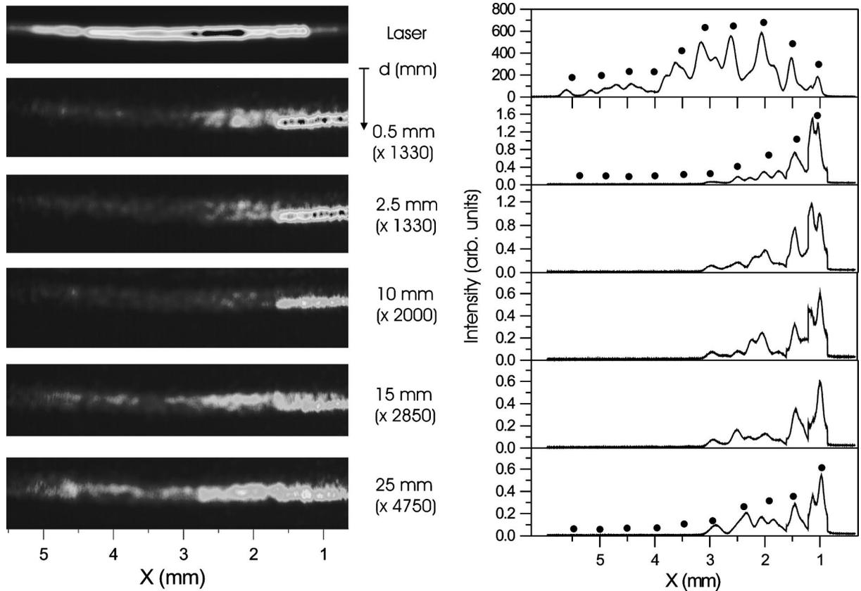
FIG. 2. Left: streak camera measurements as the optical fiber separates from the sample. The top panel is the beam picture without sample. Note that the intensity spreads slowly as  $d$  is increased. The numbers at the side scale the intensity. Right: digitized transversal cut of the intensity distributions displayed on the left. The intensities for the sample are normalized to the incident intensity (top panel) and the thick dots represent the position of each fiber [see Fig. 1(a)].
