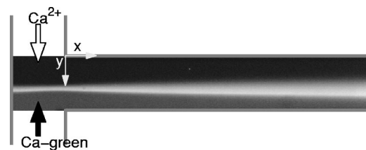
FIG. 3. Fluorescent microscopy image of the binding of \text{Ca}^{2+} ions with Calcium-Green marker in a T channel. The channel width is 200 \mu\text{m} , and the depth is 10 \mu\text{m} . Here, the velocity in the main channel is U = 0.083 \text{ cm/s} .
