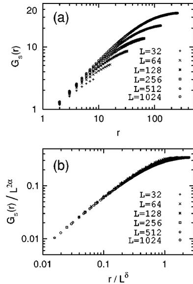
FIG. 2. The height-height correlation functions for  $u=1/2$  in the saturated regime ( $t \gg L^{z'}$ ). (a)  $G_s(r;L)$  for the systems of sizes  $L=32, 64, 128, 256,$  and  $512$  are shown in logarithmic scale. (b) The rescaled height-height correlation function  $G_s(r;L)/L^{2\alpha}$  against the rescaled distance  $r/L^\delta$  with  $\alpha=1/3$  and  $\delta=2/3$ .
