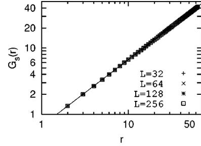
FIG. 1. The height-height correlation function for the ordinary equilibrium RSOS model with  $u=1$  [11–13] in the saturated regime ( $t \gg L^z$ ). The solid line given by  $G_s(r;L) = \frac{2}{3}r$  fits the data perfectly, indicating the wandering exponent  $\alpha' = 1/2$ .
