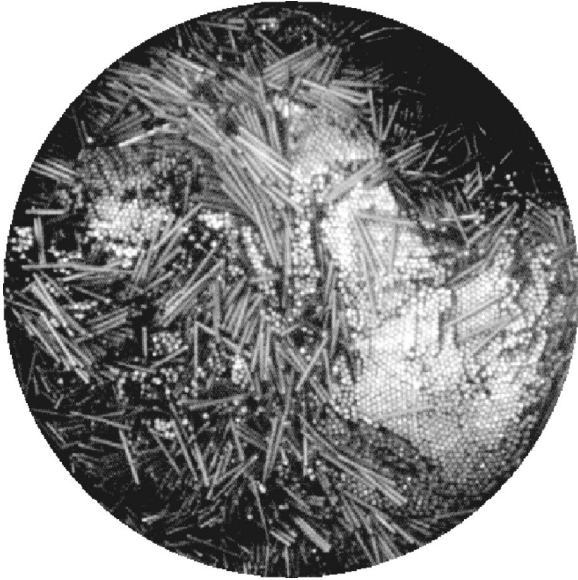
FIG. 9. Image of domains of vertical rods formed when the container is vibrated horizontally. We note that vortices are not observed. The direction of vibration is from left to right. \Gamma = 1.04 , f = 30 Hz, and n_\phi = 0.612 .
