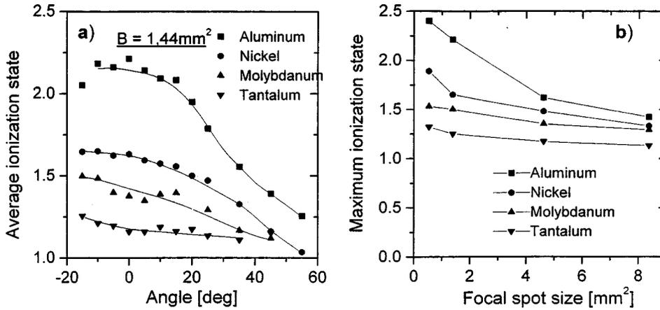
FIG. 5. (a) Angular distribution of average charge state for a fixed value of the focal spot size ( $B = 1.44 \text{ mm}^2$ ,  $I_L = 1.8 \times 10^9 \text{ W/cm}^2$ ) for Al, Ni, Mo, and Ta. (b) Maximum average charge state as a function of focal spot size for the same elements as in (a),  $E_L = 130 \text{ mJ}$ .
