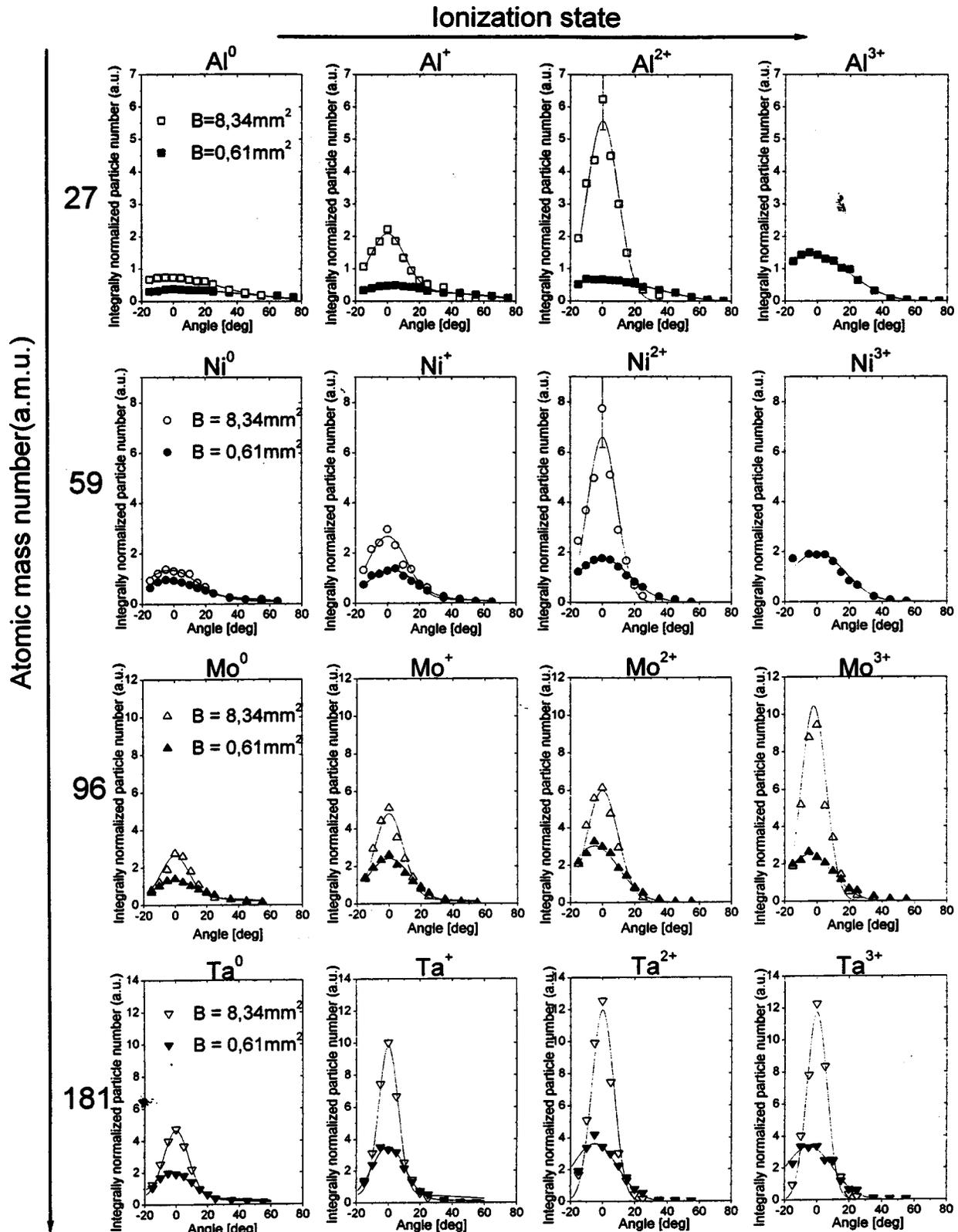
FIG. 3. Angular distribution of normalized integrated, charge-resolved particle emissions from Al, Ni, Mo, and Ta for two focal spot sizes.
