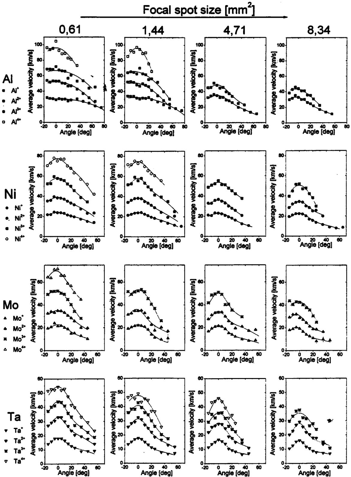
FIG. 4. Angular distribution of average charge-resolved ion velocities as a function of focal spot size (four focal spot sizes).
