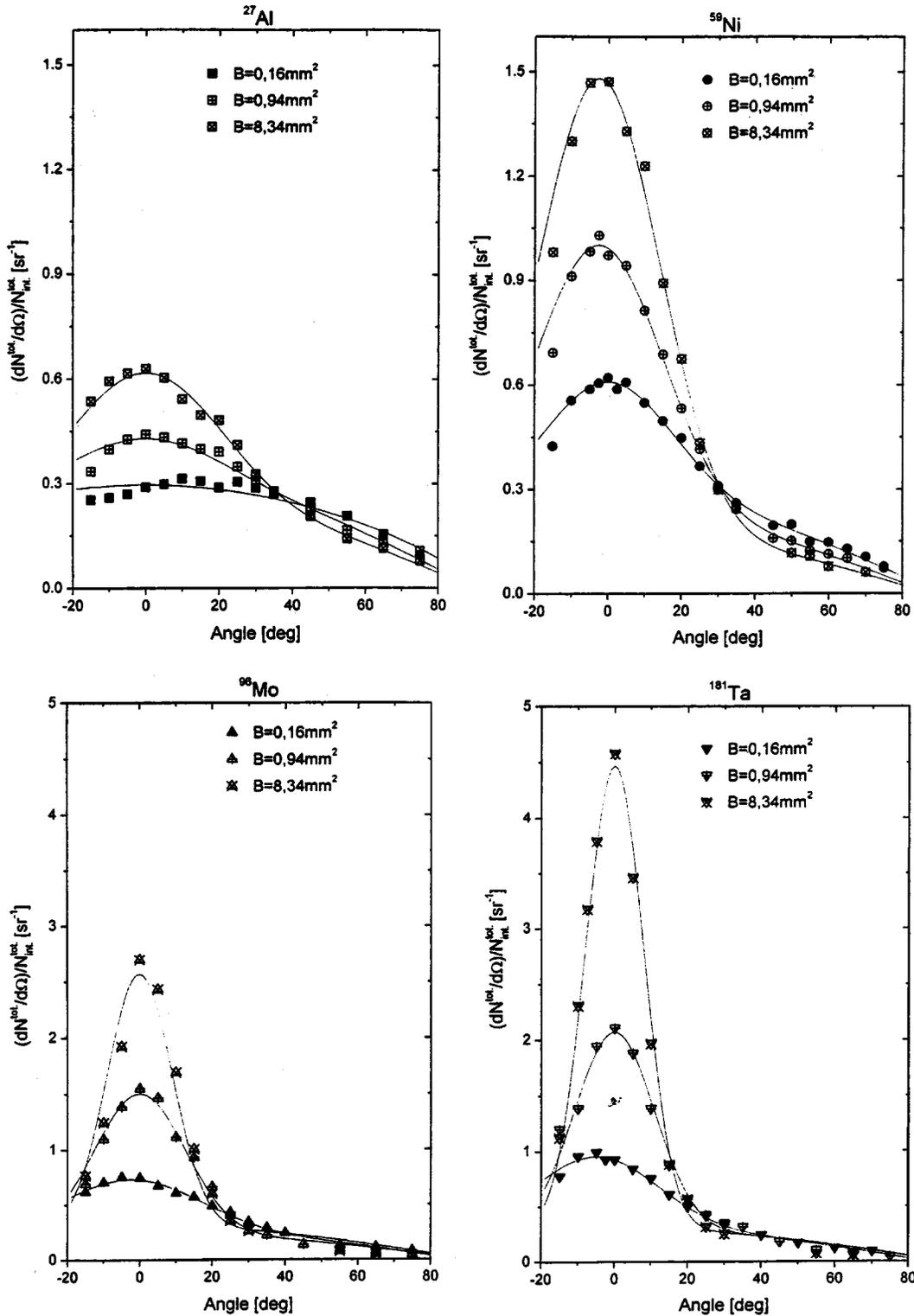
FIG. 2. Angular distribution of normalized integrated emissions from Al, Ni, Mo, and Ta for three focal spot sizes.
