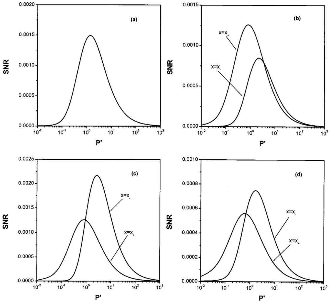
FIG. 5. SNR as a function of multiplicative noise strength  $P'$  when initial conditions are changed with different noise coupling constant  $\lambda$ . The parameters are chosen as  $\omega=0.002$ ,  $\varepsilon=0.01$ , and  $P=0.03$ . All parameters are dimensionless. (a)  $\lambda=0$ ,  $\tau_1=0.7$ , and  $\tau_2=0.2$ . (b)  $\lambda=0.5$ ,  $\tau_1=0$ , and  $\tau_2=0$ . (c)  $\lambda=0.5$ ,  $\tau_1=0.7$ , and  $\tau_2=0$ . (d)  $\lambda=0.5$ ,  $\tau_1=0$ , and  $\tau_2=0.2$ .
