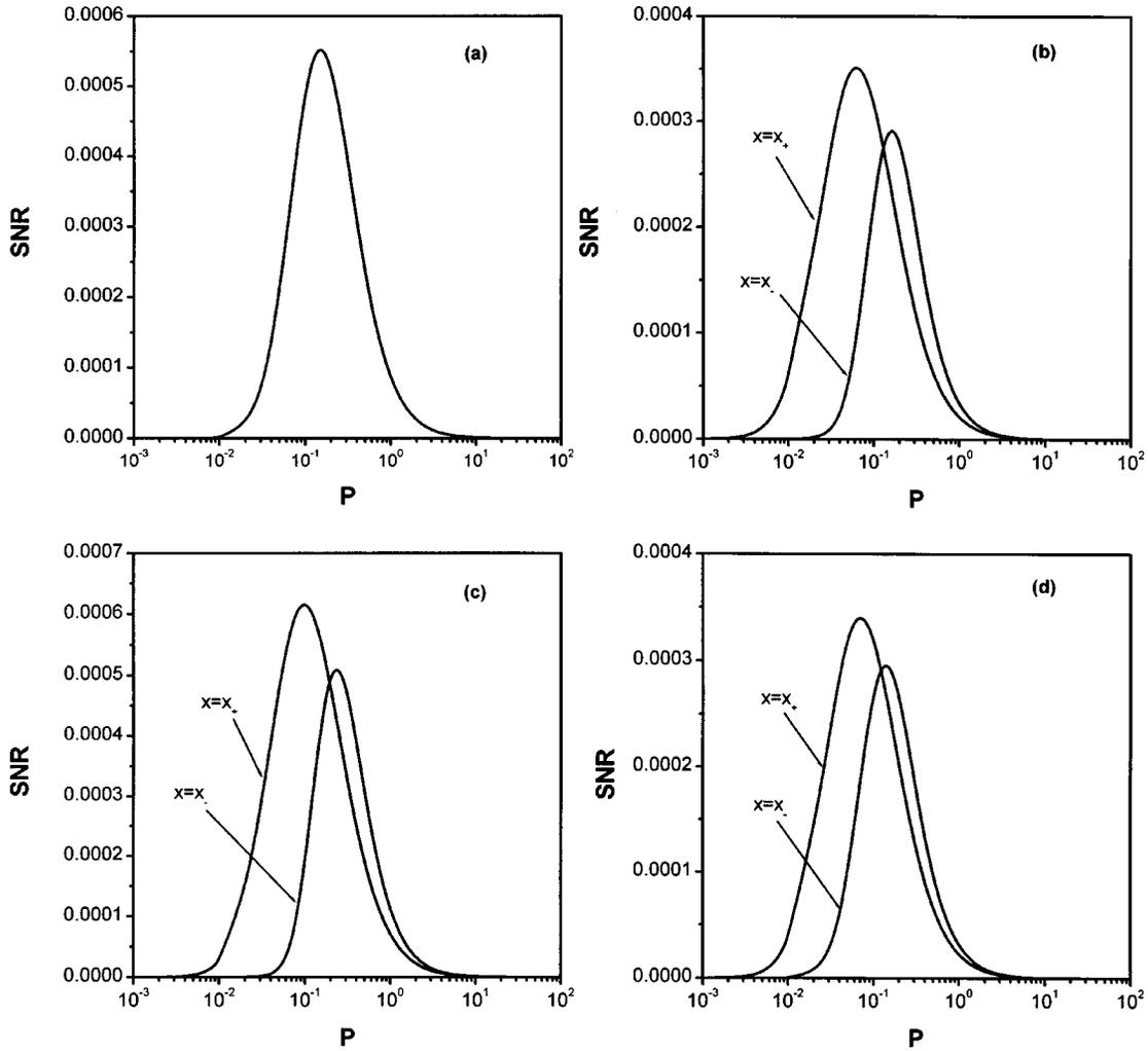
FIG. 6. SNR as a function of additive noise strength  $P$  when initial conditions are changed with different noise coupling constant  $\lambda$ . The parameters are chosen as  $\omega=0.002$ ,  $\varepsilon=0.01$ , and  $P'=0.08$ . (a)  $\lambda=0$ ,  $\tau_1=0.7$ , and  $\tau_2=0.2$ . (b)  $\lambda=0.5$ ,  $\tau_1=0$ , and  $\tau_2=0$ . (c)  $\lambda=0.5$ ,  $\tau_1=0.7$ , and  $\tau_2=0$ . (d)  $\lambda=0.5$ ,  $\tau_1=0$ , and  $\tau_2=0.2$ .
