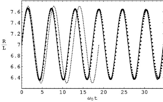
FIG. 6. Typical behavior of the plasma radius. The simulation (points) agrees with the theory (solid line). The pressureless solution (dashed line) is also shown for comparison.
