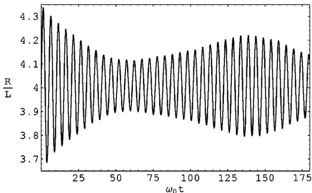
FIG. 7. The breathing oscillation for small plasmas is modulated. The present theory accurately predicts the frequency, but not the modulation.
