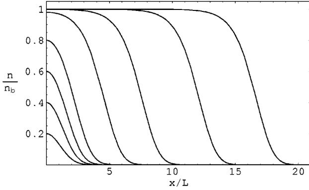
FIG. 1. Equilibrium plasma distribution  $n=n_0(x)$  versus space coordinate for different initial values  $n_0(0)/n_b$ . As the total number of particles increases or the temperature decreases the Gaussian density profile gradually changes to a step profile.
