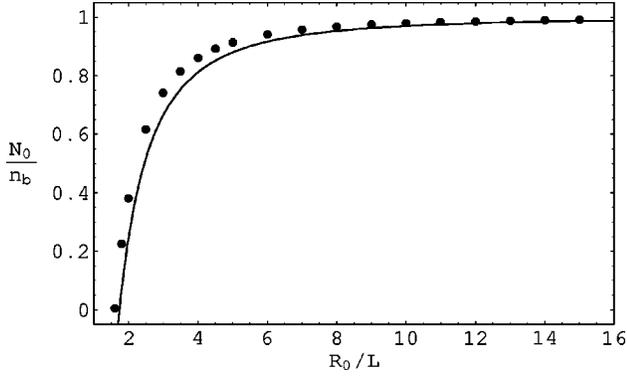
FIG. 3. Equilibrium plasma density versus slab dimension. The result from Eqs. (5) and (6) (points) is in good agreement with that of Eq. (17) (solid line).
