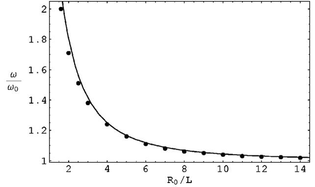
FIG. 8. Frequency of plasma oscillations versus slab dimension. The simulation result (points) is in good agreement with that of the theory (solid line).
