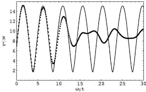
FIG. 9. The half size of the plasma cloud versus time for a solution with  $a > 1$  from theory (solid line) and simulation (points). Such a solution would inevitably blow up in the cold-plasma limit. Pressure accounts for the regular plasma behavior observed here, whereas the apparent instability is not described by the present theory.
