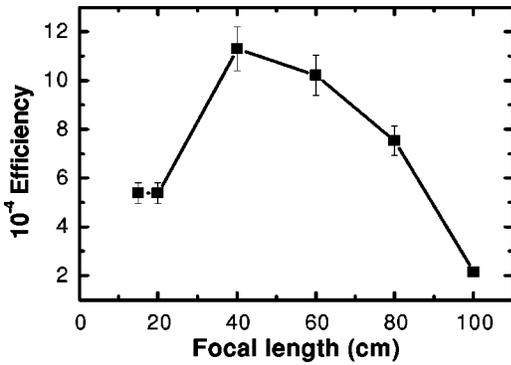
FIG. 4. The conversion efficiency between the fundamental wave and the TH versus focal length of the lens.
