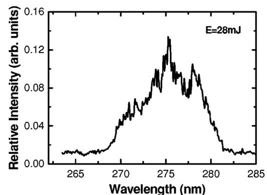
FIG. 3. The spectra of the TH with a fundamental wave laser energy of  $E=28$  mJ and a lens with a focal length of  $f=40$  cm.
