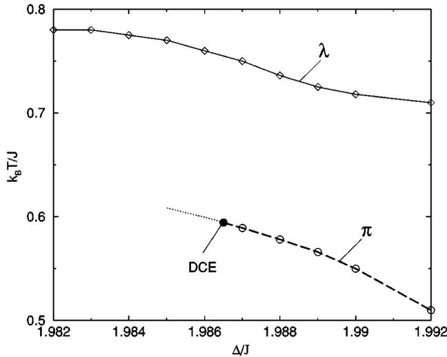
FIG. 2. Portion of the  $S$  surface phase diagram of Fig. 1 close to the DCE (in the reduced variables  $\Delta/J$  and  $k_B T/J$ ). Diamonds represent the second-order  $\lambda$  phase transition line. Circles give the first-order  $\pi$  transition line (the dashed line is a guide to the eyes). The finite-size extension is given by the dotted line. The filled circle indicates the position of the DCE. Errors do not exceed the symbol sizes.
